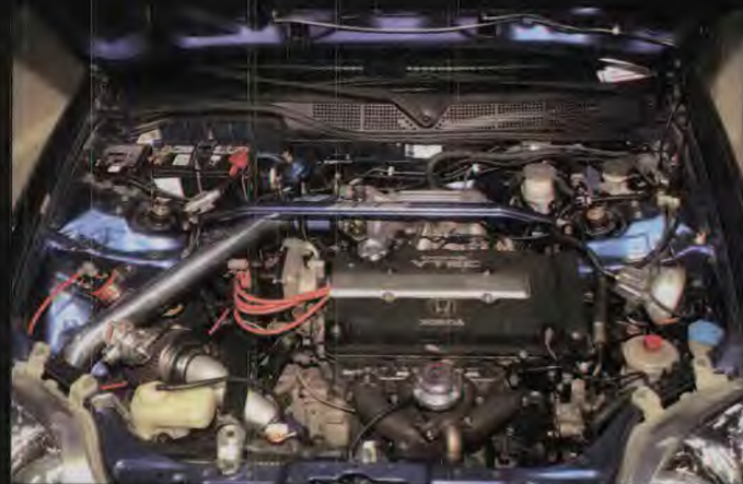
Under the hood of Cpl. Brad Sanders’ 2000 Honda Civic Si is a four cylinder turbo charged engine equipped with large fuel injectors, performance enhancing computer chip and various other performance improving parts.
