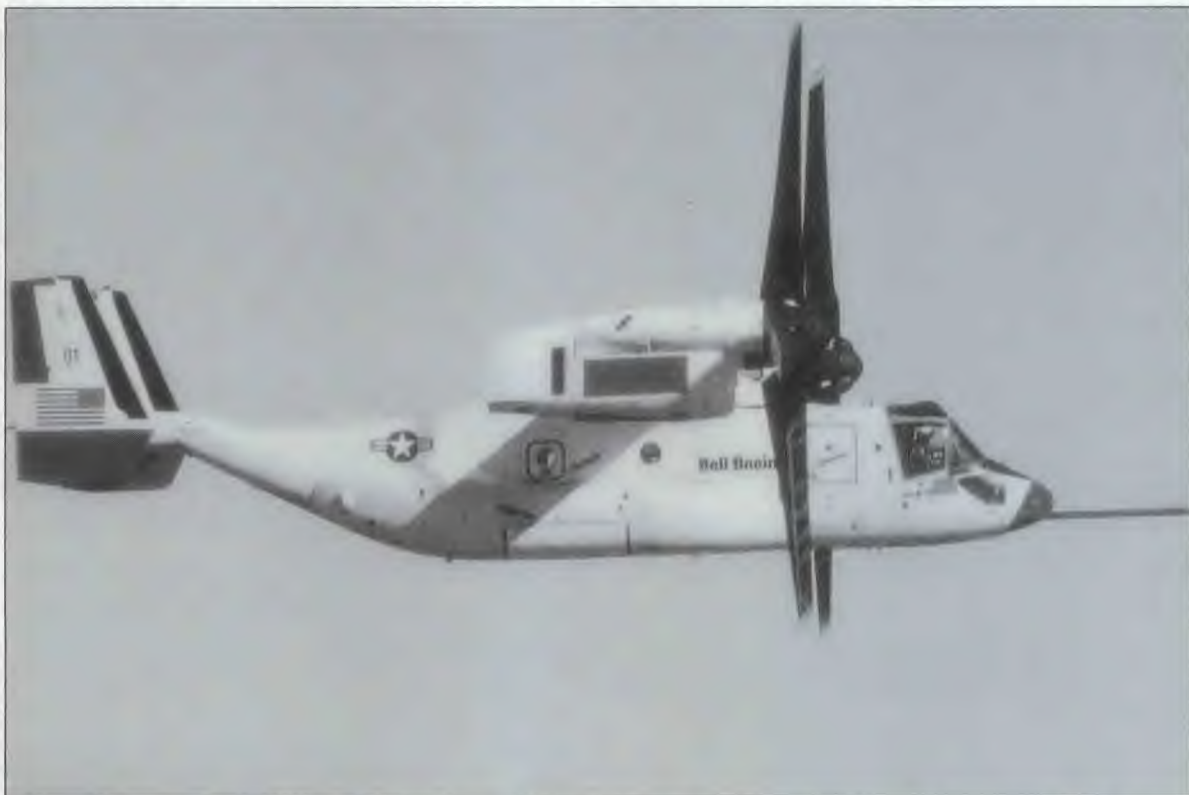
The V-22 Osprey flies like a turboprop airplane. It possesses greater speed and range than today's helicopters and can land and take off vertically.
