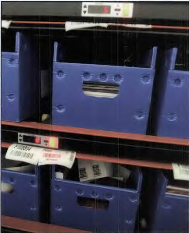
The shipping run begins with the Pik-2-Lite system, which sorts processed Marine Corps Institute textbooks into coded bins and indicates how many of each book are on order. Only one Marine is required to operate this system, which gives the Marines more time for other operations and training.
