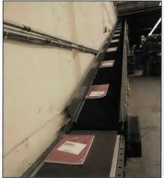
The 359 ft. conveyor belt ascends high into the Marine Corps Institute warehouse, allowing clearance for the forklift to operate underneath. The belt then descends into the postal section, where automated rollers sort books into mailing bags for shipment.
