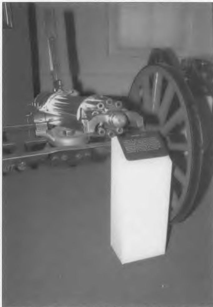
The Gatling Gun, invented in 1862 by Dr. Richard J. Gatling, a dentist, was the first practical machine gun. This one is an 1865 model, and was mounted on an 1871 naval landing carriage. (photo by Cpl. Matt S. Schafer)
